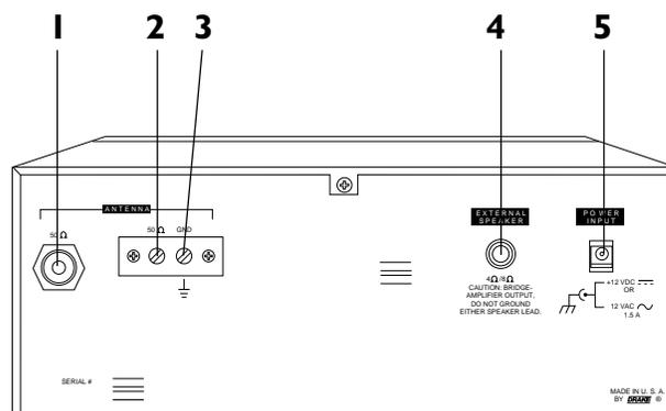
**1) 50 Ohm SO-239 Connector** - This antenna input is a 50 Ohm, SO-239 coaxial input requiring a mating PL-259 connector. This input would typically be used as the primary antenna input. Antennas such as dipoles, trap dipoles, verticals and beams will provide the best results depending upon the desired receiving frequency.
