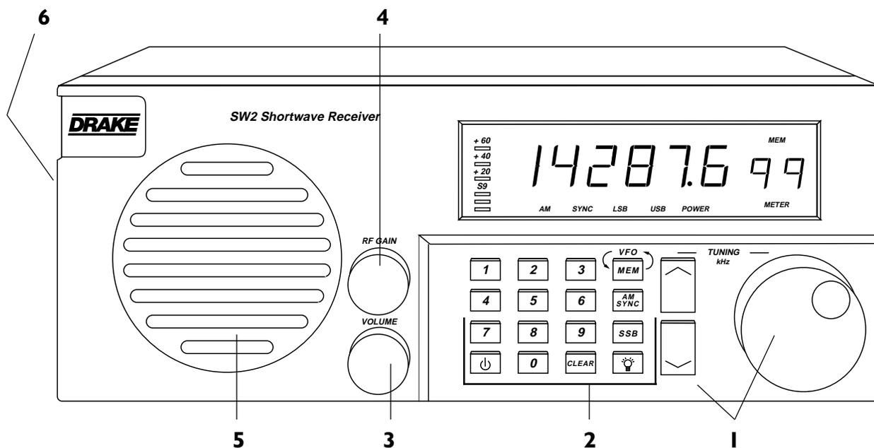
**1) Tuning (VFO)\***- The tuning wheel and the / buttons are the primary tuning controls of the receiver. Clockwise rotation of the dial increases frequency in 50 Hz steps and counterclockwise rotation decreases frequency in 50 Hz steps. The / buttons increment and decrement the frequency in 5 kHz steps. Press and hold the or and the rate of 5 kHz steps will increase. \*The VFO (Variable Frequency Oscillator) represents the normal tuning mode of the receiver.
