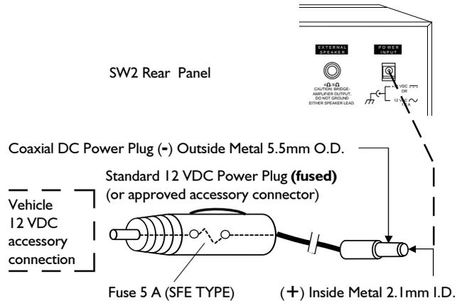
**FIGURE 1 - PROPER WIRING POLARITY AND FUSING DIAGRAM**
