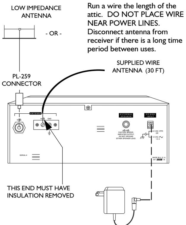
**FIGURE 2 - BASIC ANTENNA CONNECTIONS**
