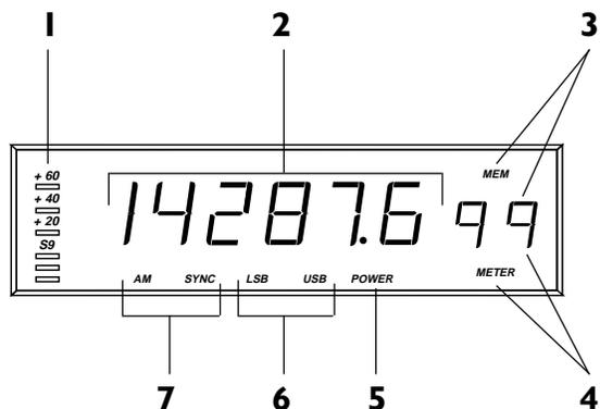
**1) Bar Graph** - This bar graph display indicates the relative received signal level in S-units and dB above S9.
